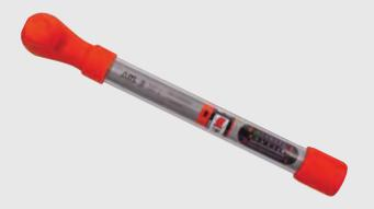
Using injection moulded Nylon 11, Norbar's insulated torque wrench complies with IEC 60900:2004 and is more durable than the traditional PVC dipped insulated tools. Certified to 1000 volts.
