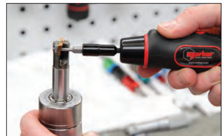
Bit holder can be removed and replaced with widely available screwdriver blades.
