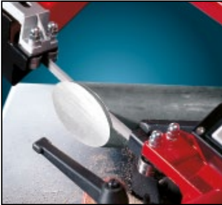
Wide cutting performance 105 mm with adjustable left cutting angle from 0° to 45°.
